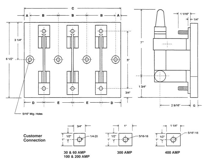
NOTE: 30 and 60 Amp - Parts bright dipped, insulation red polyglass 100 to 400 Amp - Parts silver plated, insulation red polyglass
