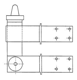
Type B Heavy Duty Knife Switches are similar to Type A, except they are back connected units without base plates. The 30, 60, 100, 200, 300 and 400 amperes sizes utilize stud connections. The 600 ampere and larger sizes utilize bus bar connections.
