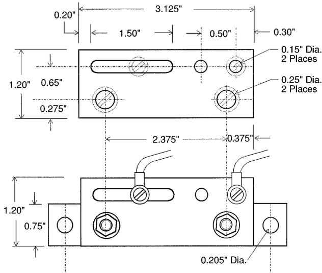
Tolerances  $\pm .015$  for the hole diameters. Other tolerances  $\pm .030$  unless specified. Dimensions subject to change without notice.
